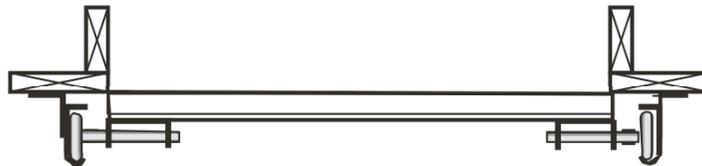
Verify that the superior extremities of the rails are at the same level. After verifications and adjustments, the following step is to definitely fix the rails in place, respecting the distance of half an inch ( $\frac{1}{2}$ " ) on the bottom and of half an inch ( $\frac{1}{2}$ " ) on the top, between the panels and the rails. Make sure that the rails are at level.
